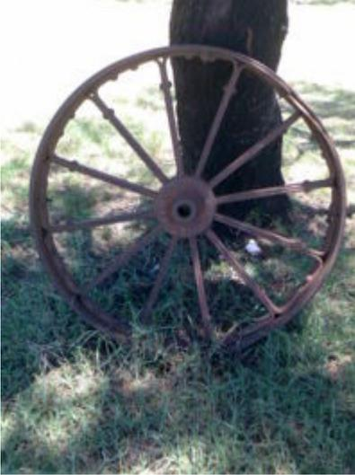
Metal [wheel](#) with riveted spokes and tyre.
